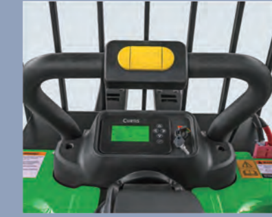
The CURTIS AC Control System
