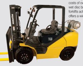
This family of 8,000 thru 11,000 lb. capacity pneumatics achieves its durability and low costs of ownership from its rugged designs and field proven components. With standard wet disc brakes and a Closed-center Load Sensing hydraulic system (CLSS) these forklifts achieve reduced costs of operation and reduced maintenance costs. This family offers a wide range of models to handle a wide variety of demanding applications.
