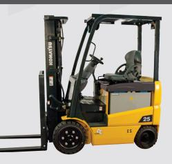
This family of four wheel electric sit-down riders boasts 36/48 volt TOTAL AC electrical system and extreme energy efficiency for long run times and very low cost of operation. Available in 4,000 thru 6,500 lbs. capacity.
