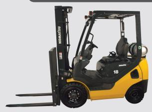
This family of engine powered, pneumatic tire forklifts delivers power and performance. With a standard 2.1 liter, EPA compliant engine and field proven components, this compact and powerful forklift can handle the toughest applications with ease. Available in 3,000 and 3,500 lb. capacities.
